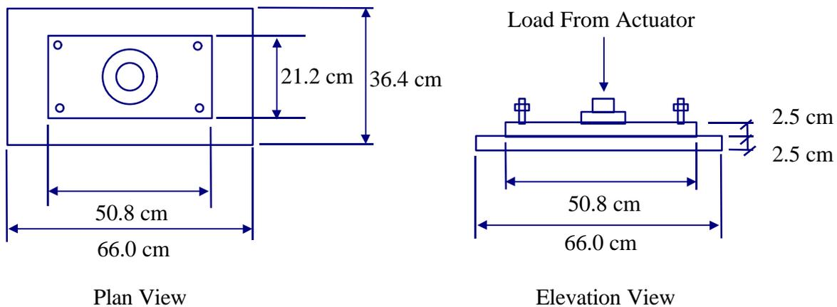
**Figure 14. Illustration of Load Plates and Connections**
