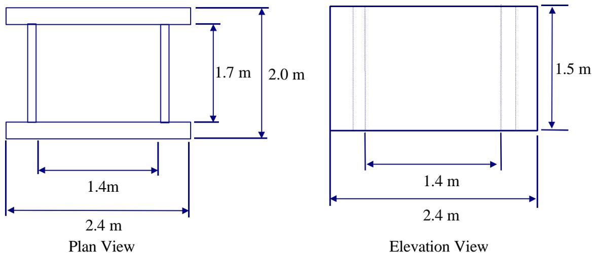
**Figure 11. Dimensions of Concrete Testing Chamber**
