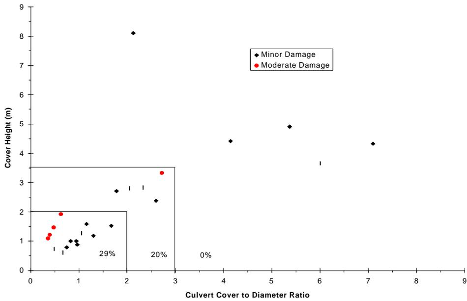
**Figure 9. Cover Height versus Cover Ratio, Pine Haven Road**
