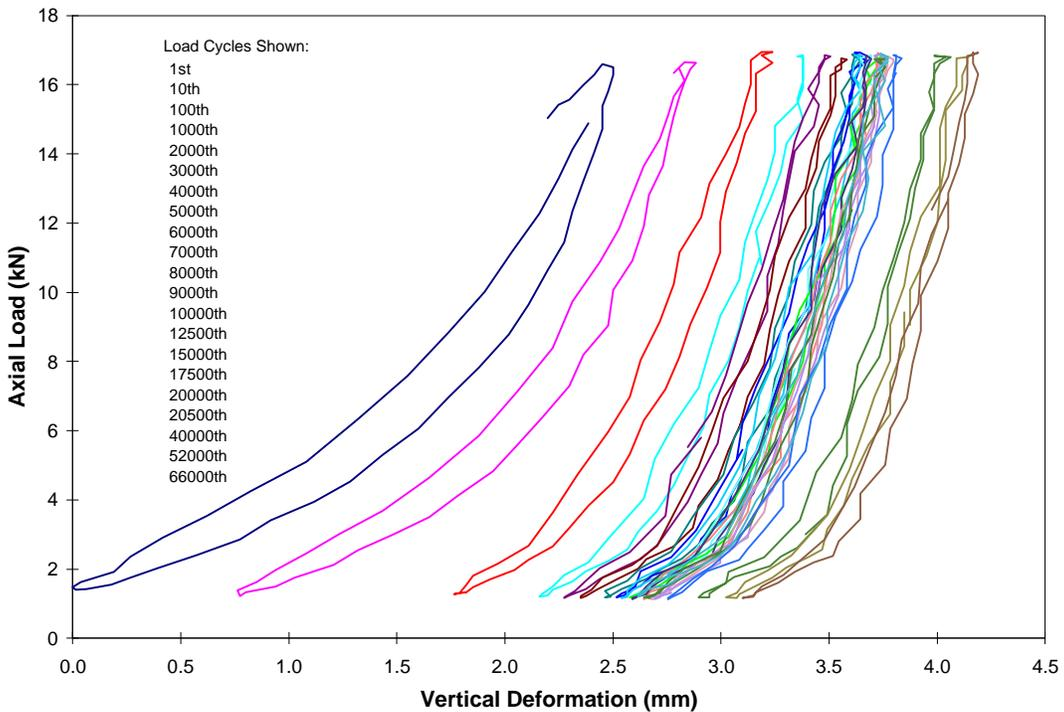
**Figure 22. Test #4 Tensar BX1100 Geogrid Load vs. Deformation for Increasing Cycles**
