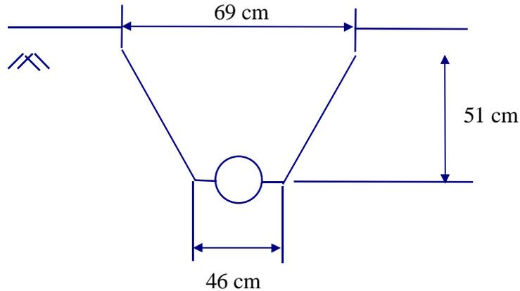
**Figure 13. Excavated Trench for CLSM Backfill.**
