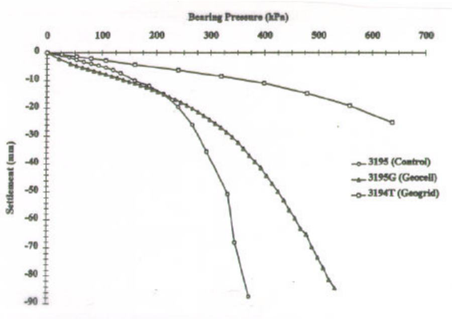
**Figure 4. Typical Bearing Pressure vs. Settlement Curve (Adams and Collins 1997)**
