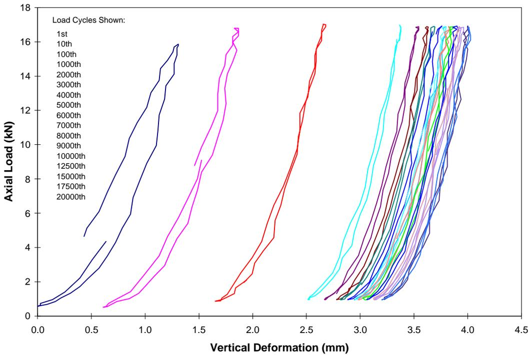
**Figure 24. Test #5 Unreinforced Sand Load vs. Deformation for Increasing Cycles**
