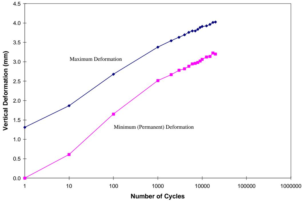
**Figure 23. Test #5 Unreinforced Sand Deformation vs. Number of Cycles**
