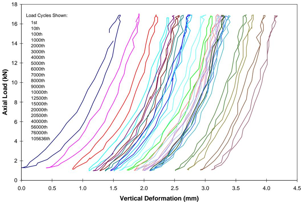
**Figure 20. Test #3 Unreinforced Clay Load vs. Deformation for Increasing Cycles**
