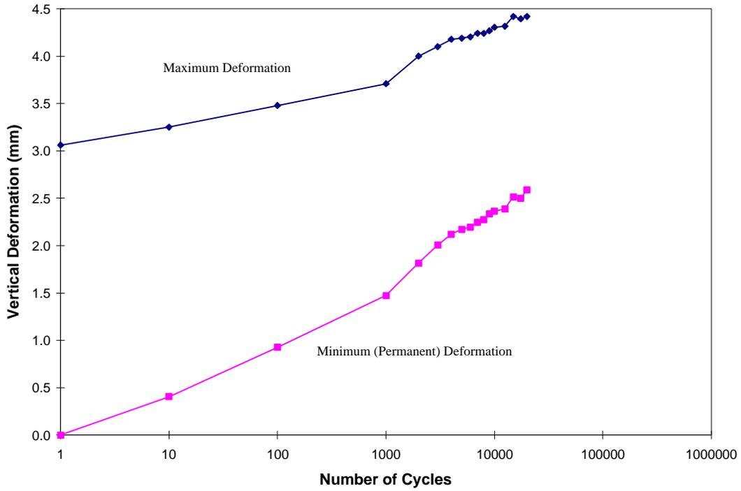
**Figure 25. Test #6 Tensor BX1300 (SS-3) Geogrid Deformation vs. Number of Cycles**
