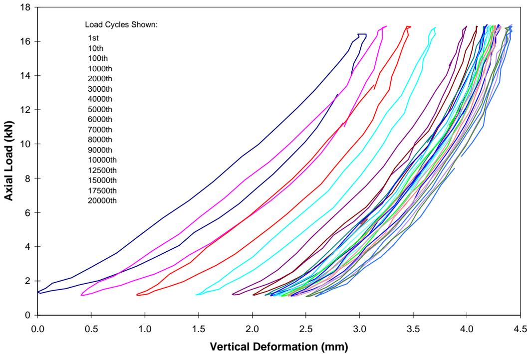
**Figure 26. Test #6 Tensor BX1300 (SS-3) Geogrid Load vs. Deformation for Increasing Cycles**
