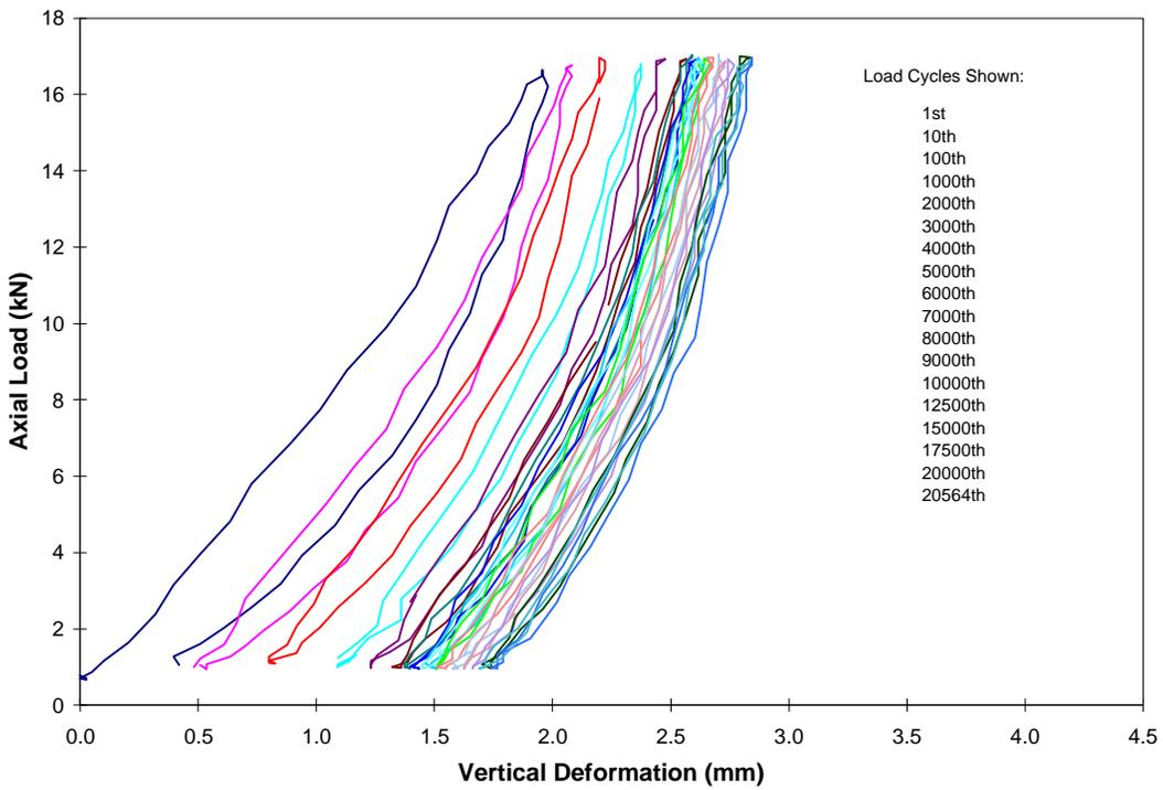
**Figure 18. Test #2 Unreinforced Clay Load vs. Deformation for Increasing Cycles**
