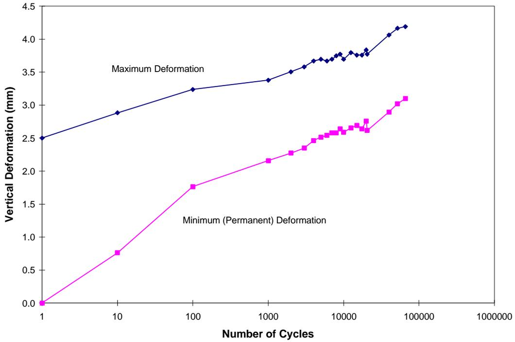
**Figure 21. Test #4 Tensar BX1100 Geogrid Deformation vs. Number of Cycles**
