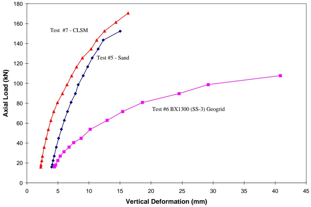
**Figure 29. Combination Plot of Load vs. Deformation for Static Loading**
