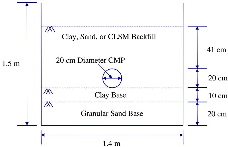
**Figure 12. Culvert Orientation and Fill Heights.**
