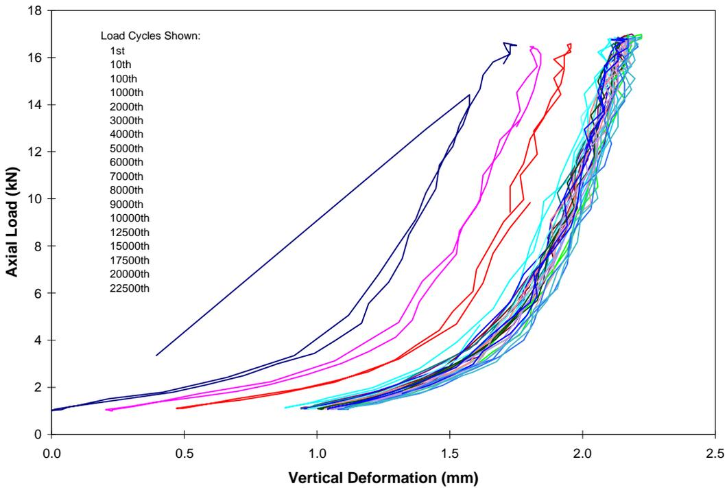
**Figure 28. Test #7 CLSM Load vs. Deformation for Increasing Cycles**
