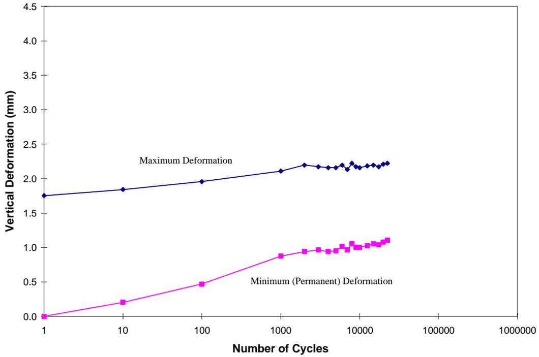
**Figure 27. Test #7 CLSM Deformation vs. Number of Cycles**
