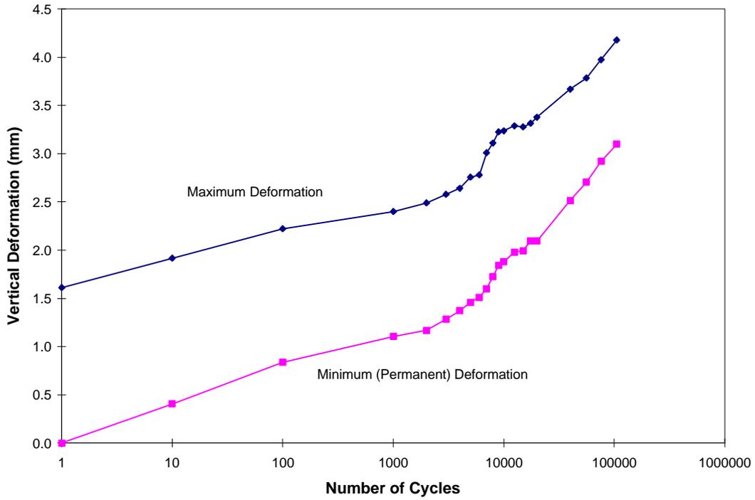
**Figure 19. Test #3 Unreinforced Clay Deformation vs. Number of Cycles**
