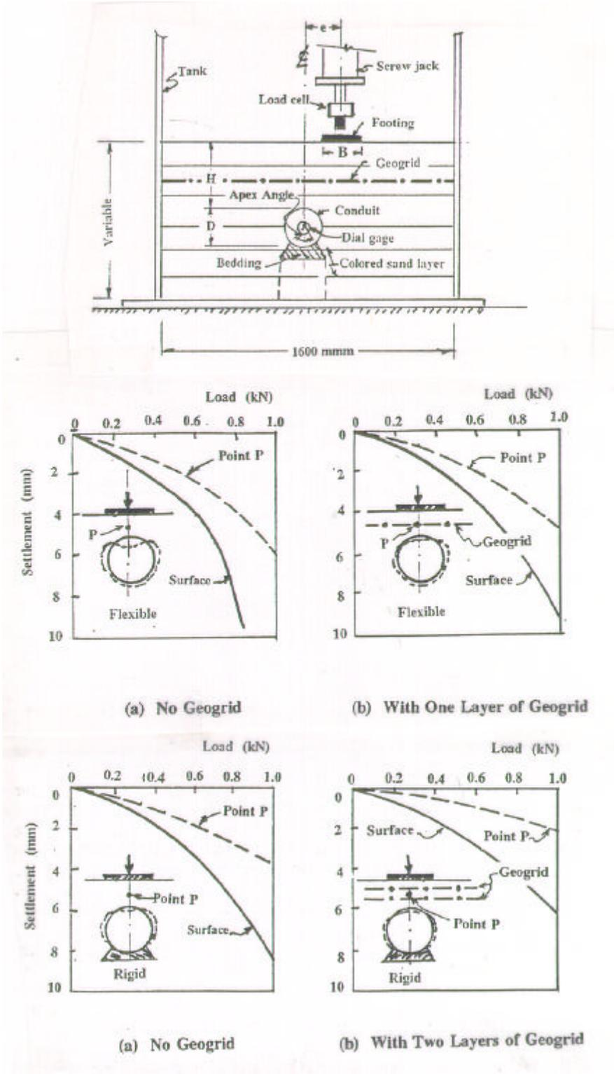
Figure 3. Test Setup and Load-Settlement Responses (Bauer 1994)
