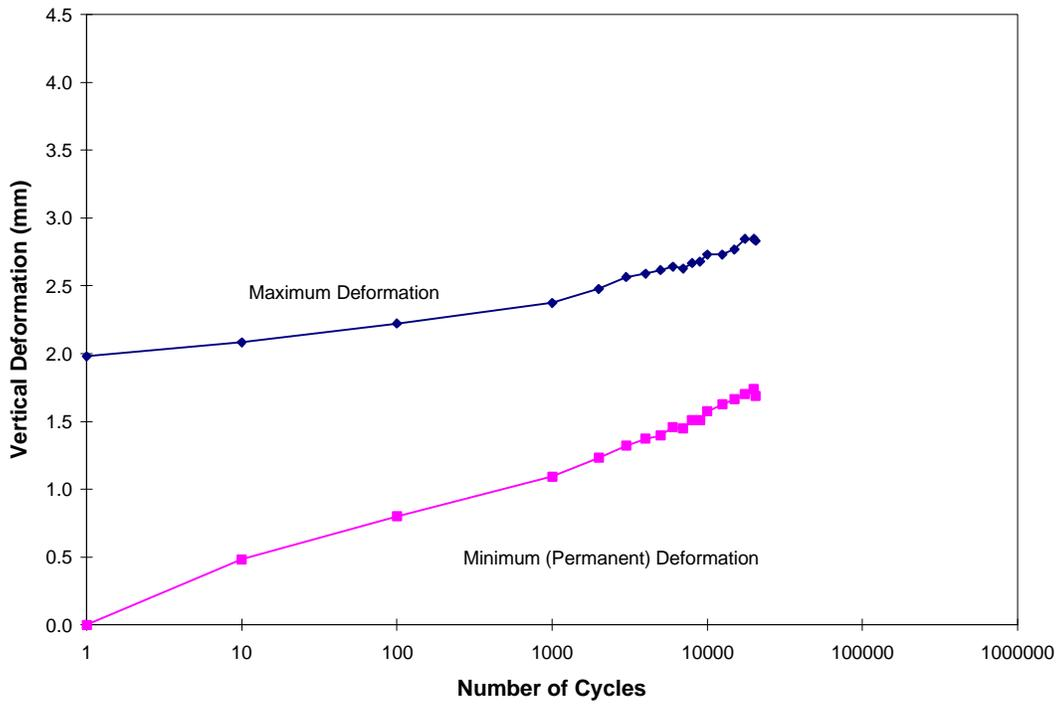
**Figure 17. Test #2-Unreinforced Clay Deformation vs. Number of Cycles**
