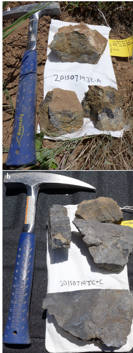
Figure 14. Samples of phosphate rock from the North Fork of Pine Creek locality. a) Sample 20150714JC-A, limonite-stained mudstone with common pisoids of apatite, and pebble-sized fragments of phosphate rock. This sample was collected from the top of the Retort Shale Member of the Phosphoria Formation. b) Sample 20150714JC-C, phosphate rock collected from float over the Meade Peak Member of the Phosphoria Formation.
