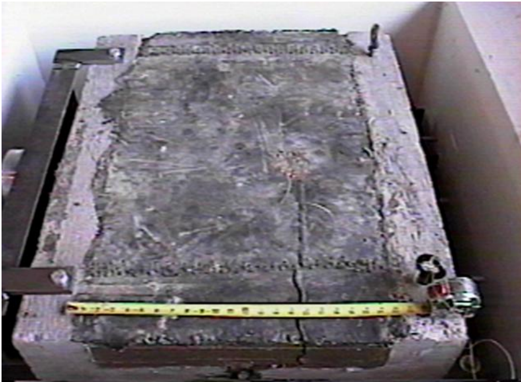
Figure 5.11 Watson Bowman Acme Failed Joint Sample.
