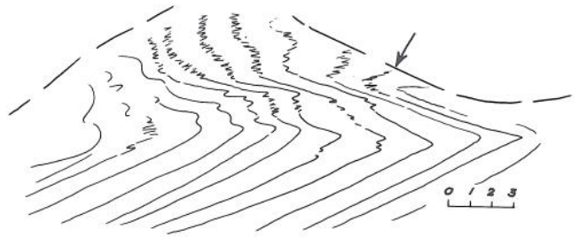
Figure 8—Deformed cross-bedding in unconsolidated sandstone generated by lateral push with board from right to left as shown by arrow Scale in inches. After McKee and others (1962, p. D155-D160).
