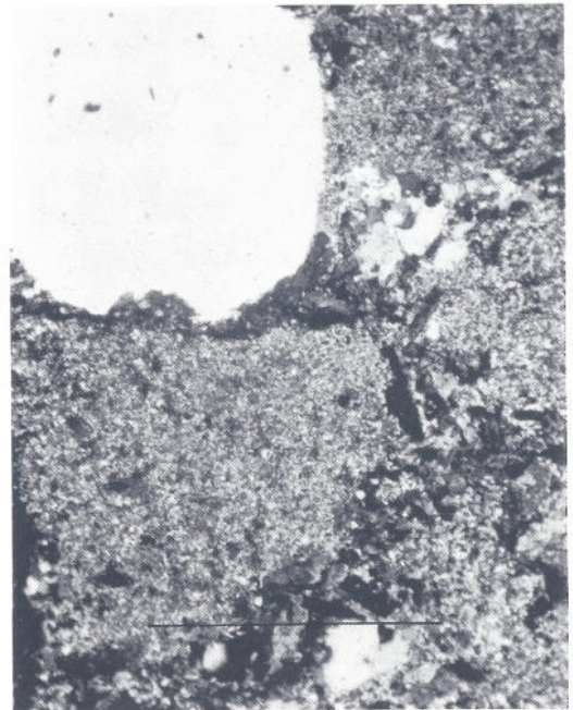
Irregular masses of chlorite schist in coarse-grained matrix of biotite-chlorite-quartz. Large euhedral crystal of quartz in upper left. Probable tuff from sec. 32, T. 18 N., R. 79 W. Line 1 mm. long.
