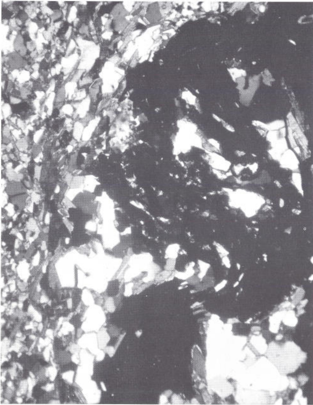
Figure 50—Photomicrograph showing folded trails of elongated quartz and opaque minerals in garnet-biotite schist southwest of Arlington, sec. 2, T. 18 N., R. 79 W. Quartz inclusions are about the same size as matrix. Trend of inclusions shows helicitic fabric at an angle to trend of schistosity shown in left. Garnet probably rotated during growth. Line 1 mm. long. A—Crossed nicols. B—Plain light.
