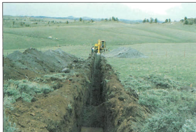
Plate 2c. Bulk sampling on the Aultman 1 kimberlite, Wyoming, by Cominco American Incorporated. Trenching of the kimberlite exposed the characteristic blue ground.
