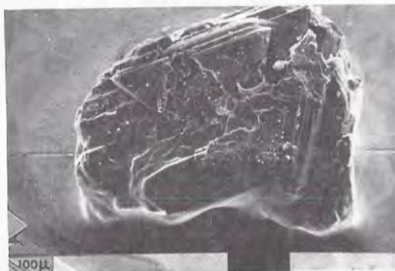
Figure 16 — SEM micrograph of flattened octahedral crystal isolated from peridotite nodule showing lamellar buildup and development of triangular shaped growth platelets on octahedral faces.
