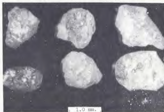
Figure 19 - Six diamonds recovered from weathered kimberlite from the Sloan 1 pipe in Colorado: total weight 14.0 mg (0.07 carat). Types are as follows: top row left to right—aggregate (SD1-X5), laminated octahedron (SD1-X6) and aggregate (SD1-X1); bottom row left to right—flat (SD1-X4), dodecahedron (SD1-X3) and irregular (SD1-X2).
