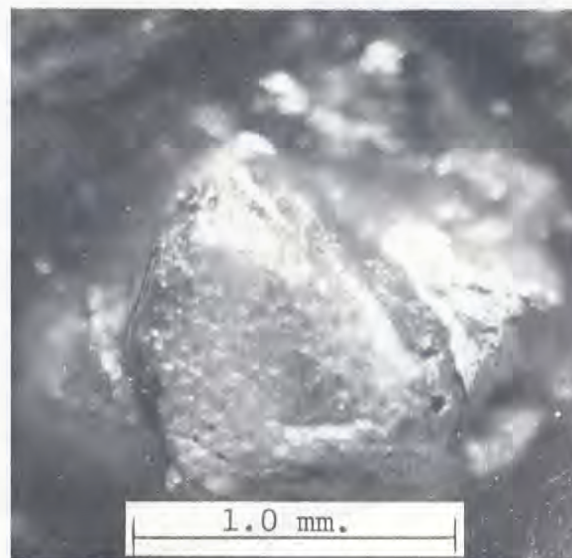
Figure 13 — Original diamond discovered during thin section preparation. It is embedded in a serpentized garnet peridotite; note rounding of edges and interpenetrant twinning.
