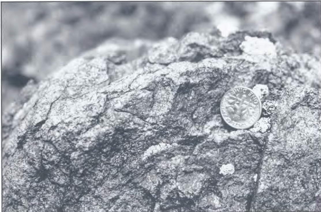
Figure 5. Cumulate-textured serpentinite from the Atlantic City mine area. Sample consists of abundant 2- to 4-mm diameter grains of serpentine after olivine and pyroxene in a serpentinitized matrix. Photograph taken at locality 23D (Plate 2).
