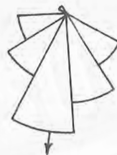
Figure 7. Rose diagram and vector mean ( \bar{x} ) for n paleocurrents in the quartzite member of the Magnolia Formation. n = 40 , \bar{x} = 191^\circ , unit vector = 0.1 inch.
