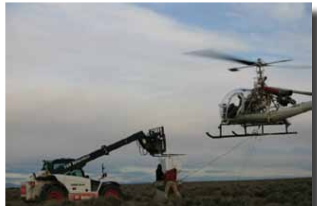
Above and below: The "Bobcat" was used to load the hopper or spreader that the helicopter used.
